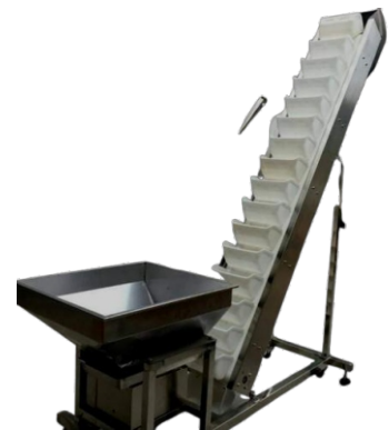
DOUGH INLET & INCLINED CONVEYOR
