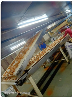
COOLING CONVEYOR 2 TIYER
